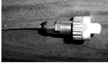
Figure 36. Woodhead Cover Placed Over RJ45 Connector
