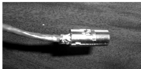
Figure 32. Metal Shell Placed Over 8-Pin DIN Connector
