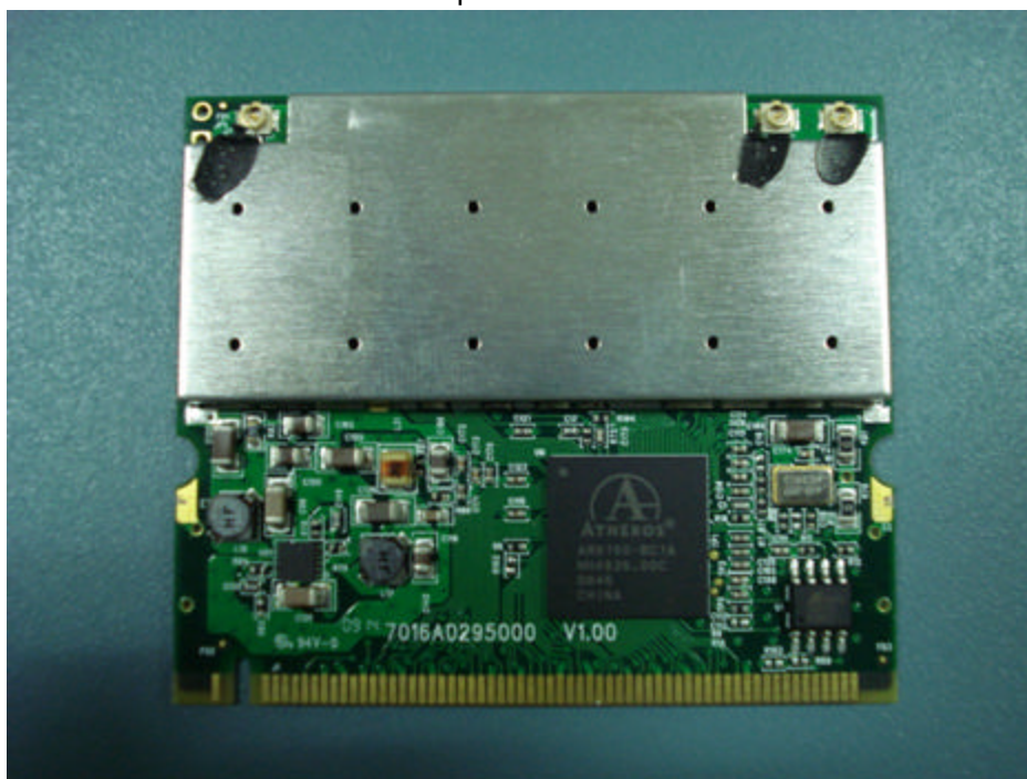
PCB with RF Module without shield – Top View
