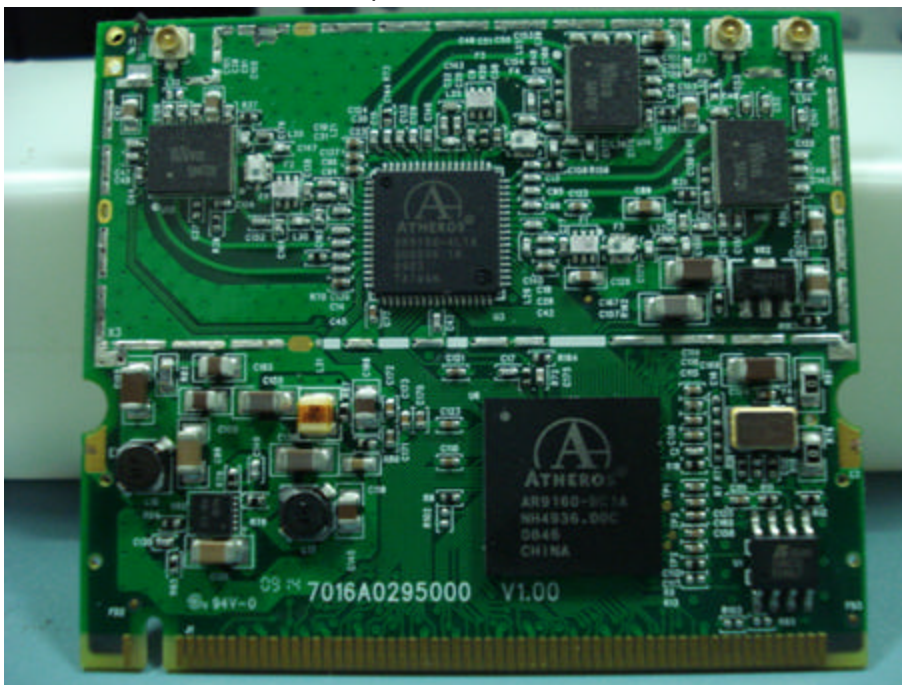
RF Module without shield – Top View
