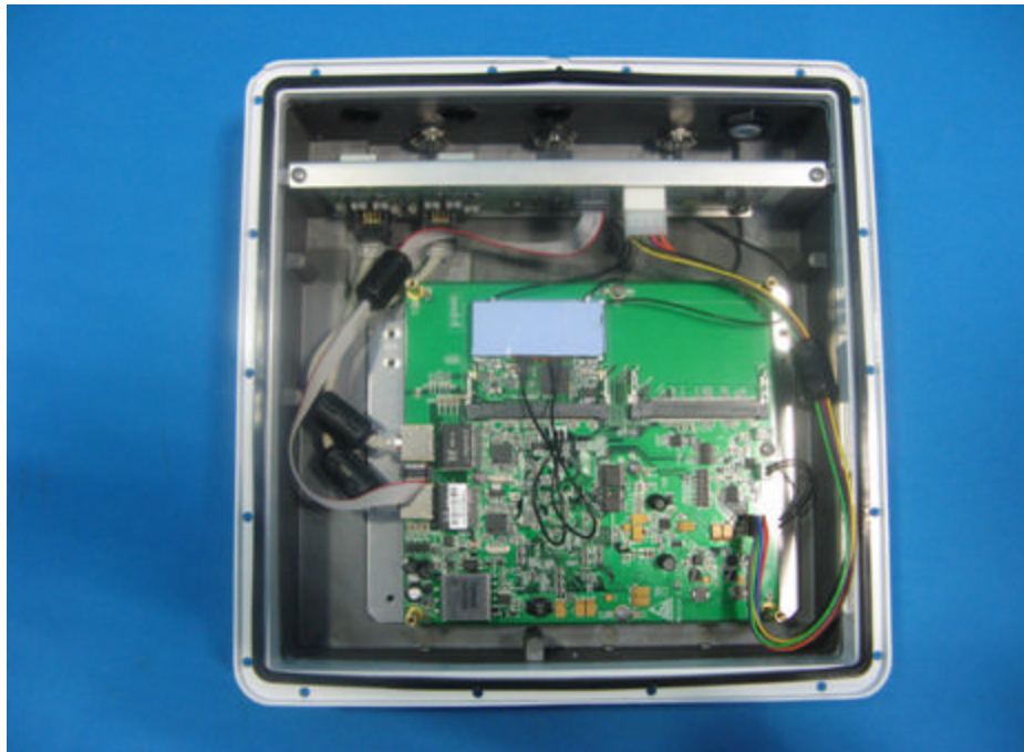
Bottom Cover – Internal View with PCB
