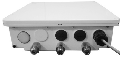
Figure 3-58 Cable Plugged In
