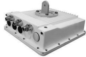
Mounting Plate fixed to the Device
