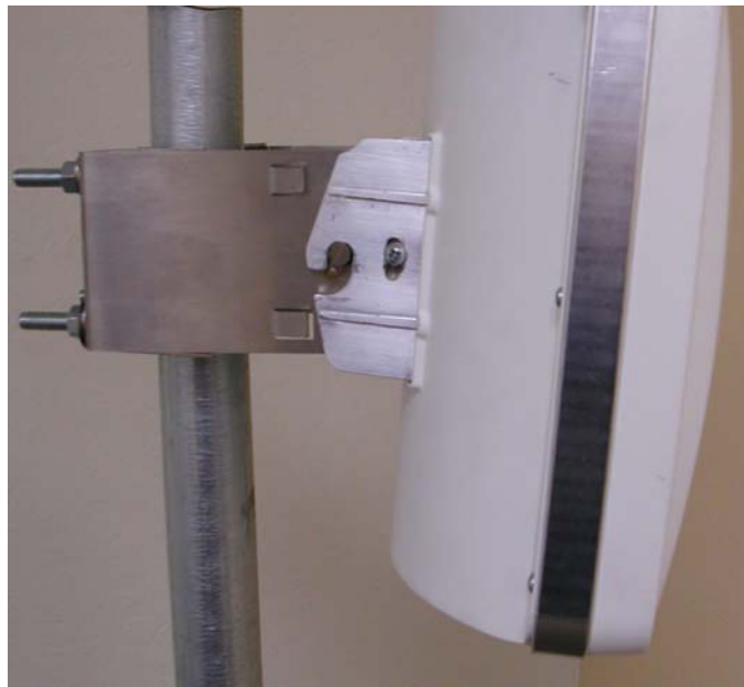
Figure 3-2: Subscriber ODU Mounting
