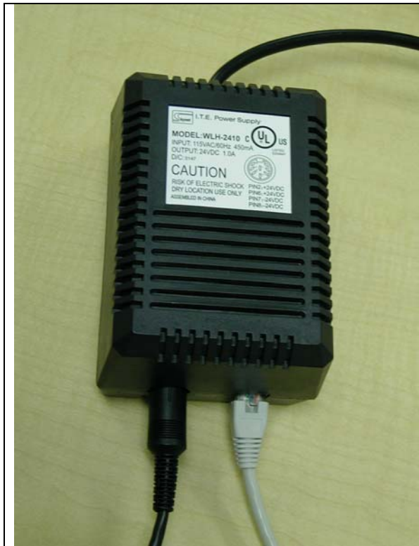
Power Brick Adapter with DIN and Ethernet
