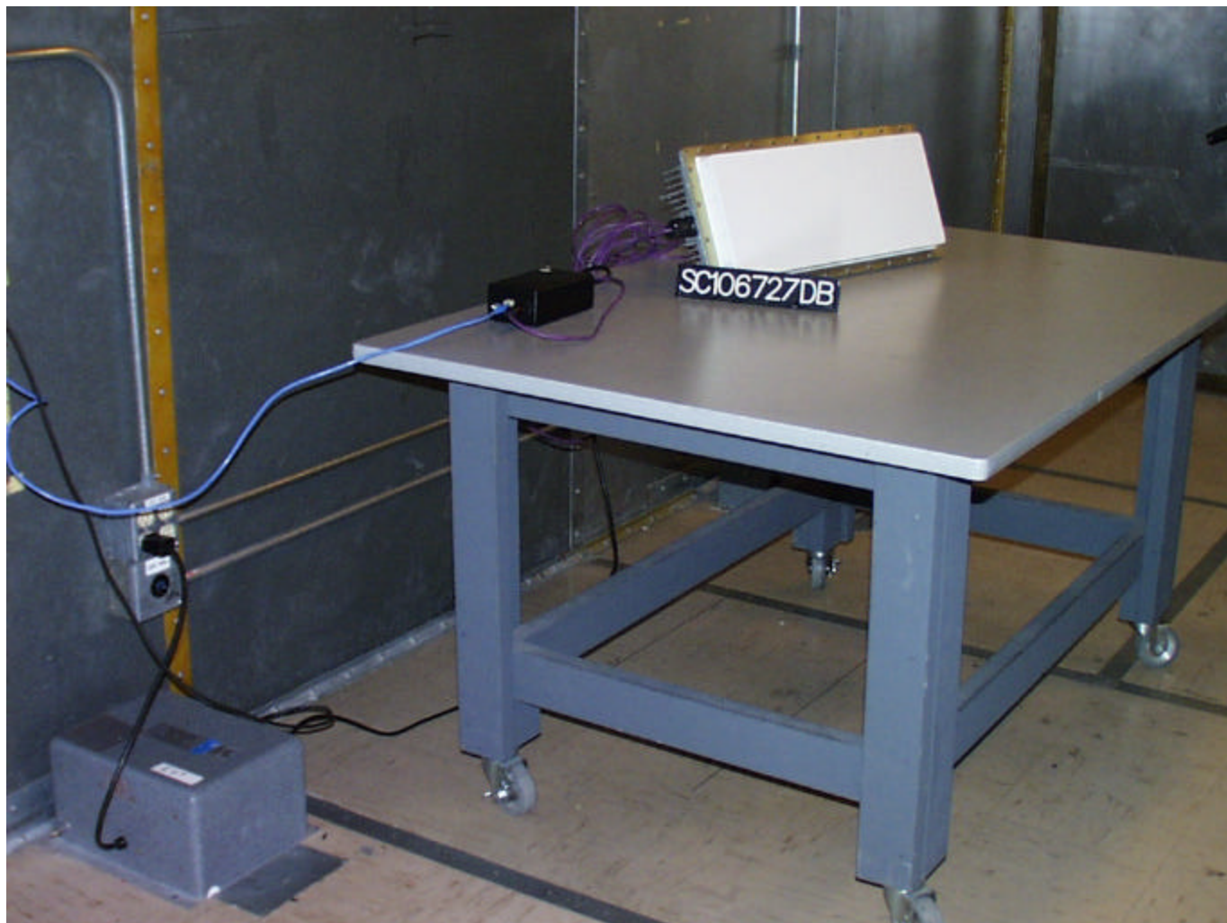
Photograph of Test Setup: AC Conducted Emission
