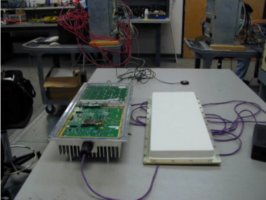
Top cover and antenna assembly removed (above).
