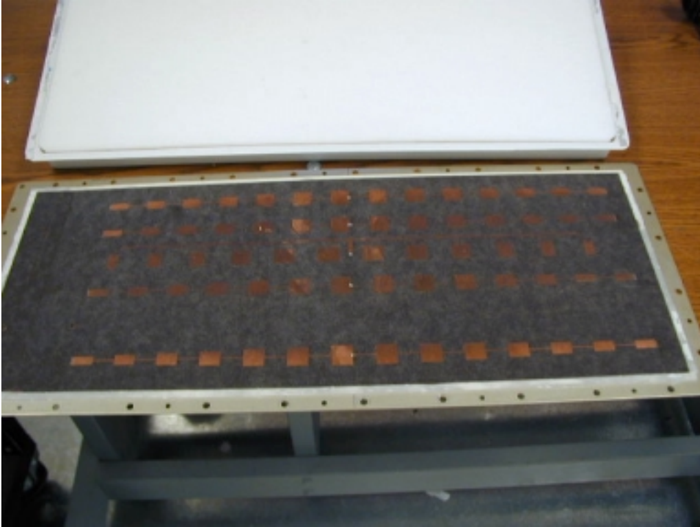
Antenna assembly, cover removed (above).
