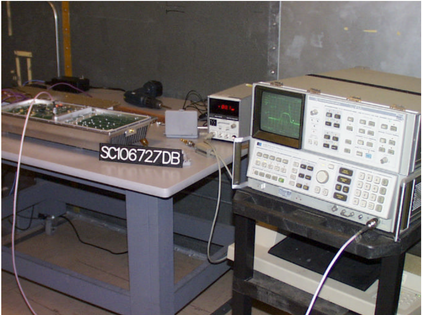
Photograph of Test Setup: Output Power and The Ratio of the Peak Excursion of the Modulation Envelope to the Peak Transmit Power
