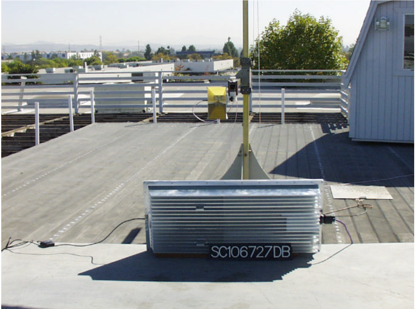
Photograph of Test Setup: Radiated Emission in Restricted Bands and Radiated Emission from Receiver L.O.
