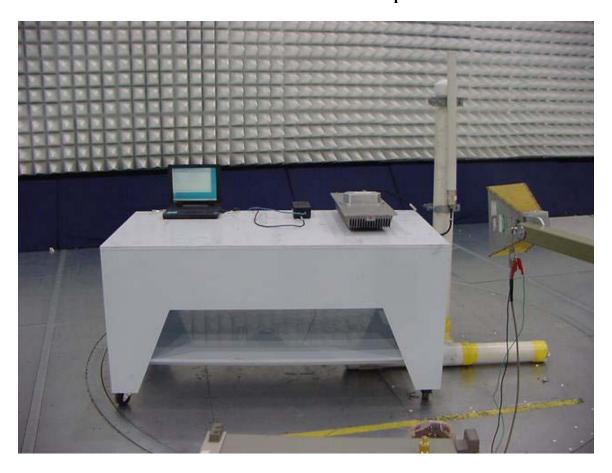
FCC ID: HZB-S58-B60C Radiated emission test setup
