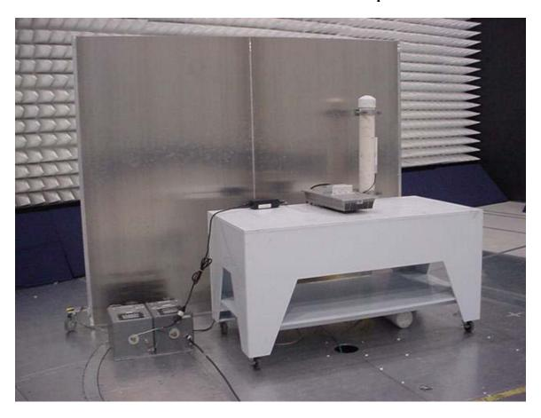
FCC ID: HZB-S58-B60C AC line conducted emission test setup
