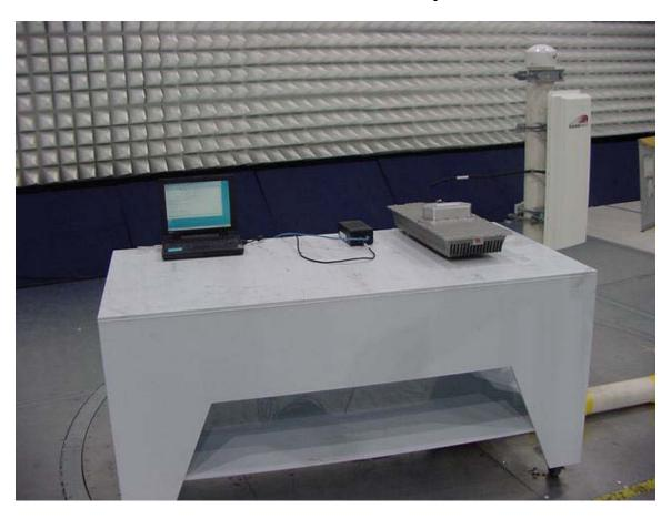
FCC ID: HZB-S58-B60C Radiated emission test setup
