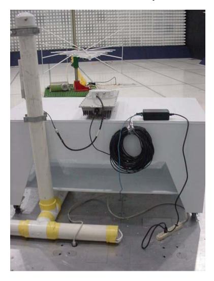
FCC ID: HZB-S58-B60C AC line conducted emission test setup
