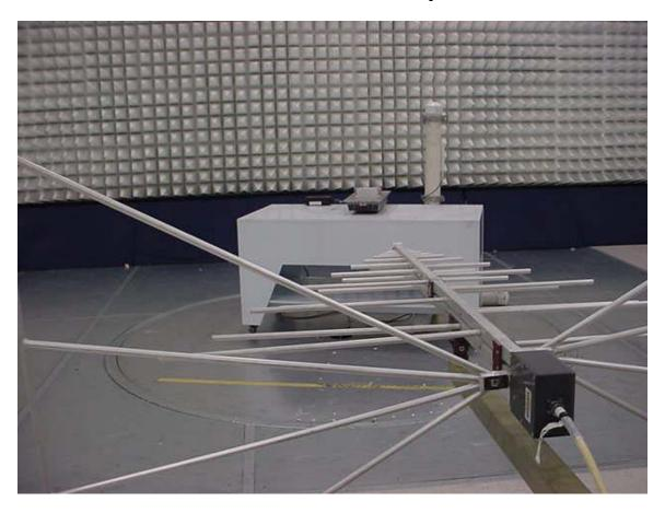
FCC ID: HZB-S58-B60C Radiated emission test setup
