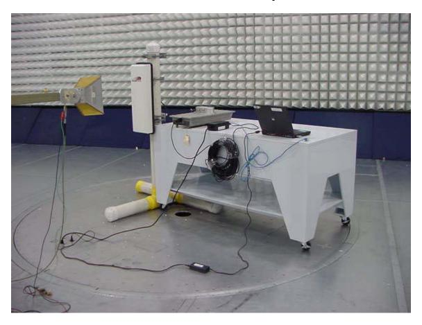
FCC ID: HZB-S58-B60C Radiated emission test setup
