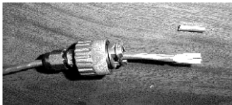
Figure 34. Cat 5 Cable with Insulation Removed
