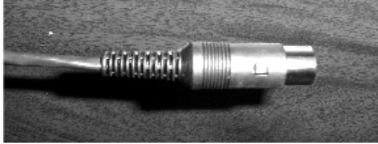
Figure 33. Jacket Placed Over 8-Pin DIN Connector
