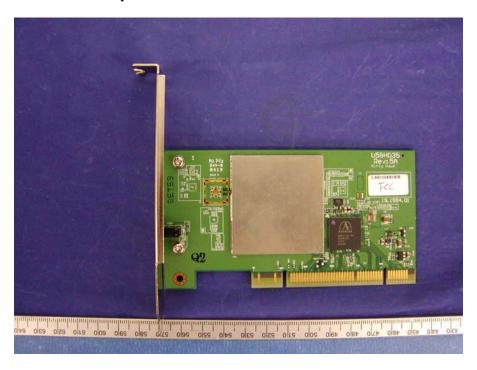
PCI Card - Component View with Shield Off
