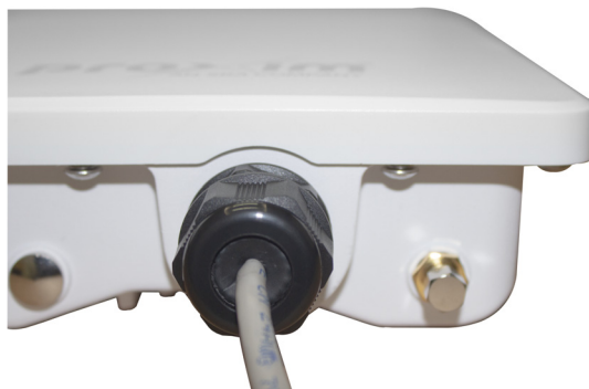
Figure 4-4 Cable Plugged In
