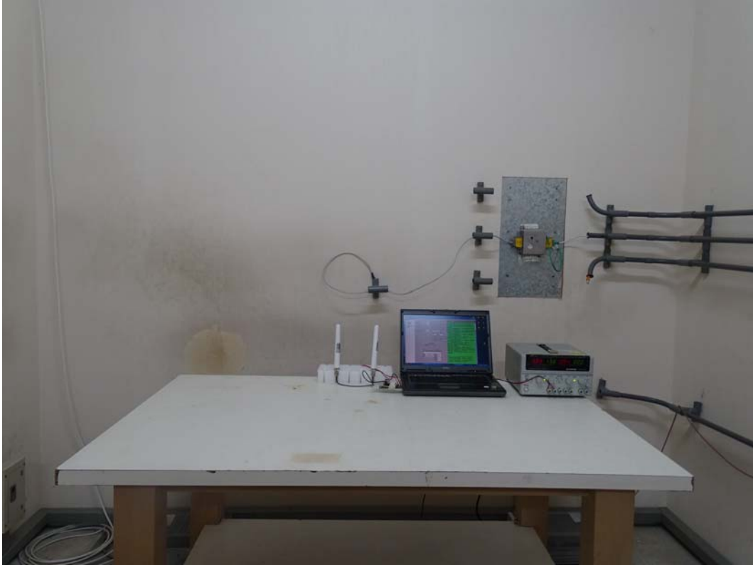
Front View of Conducted Test (Dipole Antenna)
