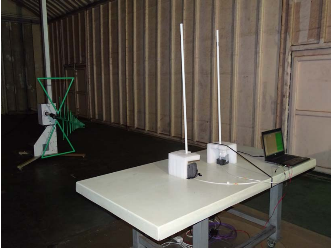
Front View of Radiated Test (Omni Antenna)
