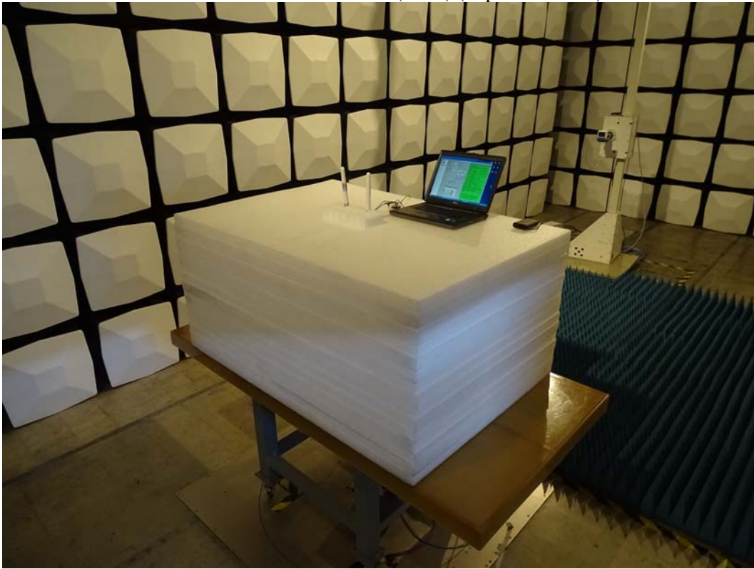
Front View of Radiated Test (Horn) (Dipole Antenna)
