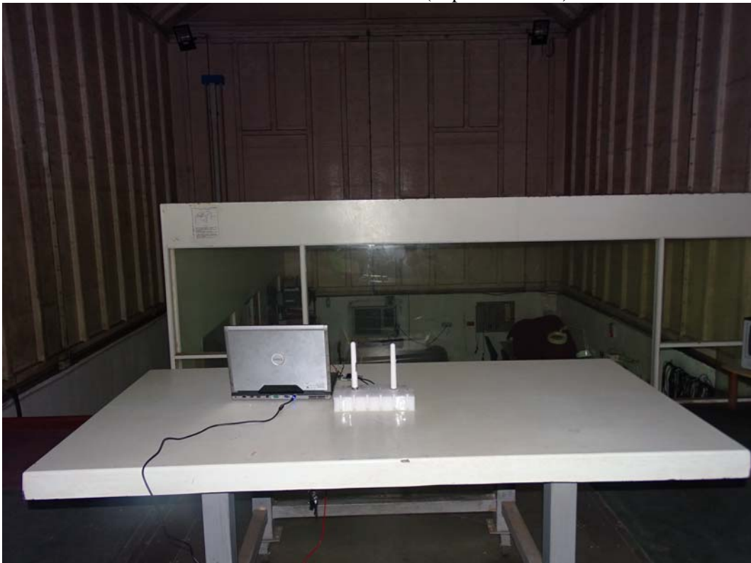
Back View of Radiated Test (Dipole Antenna)
