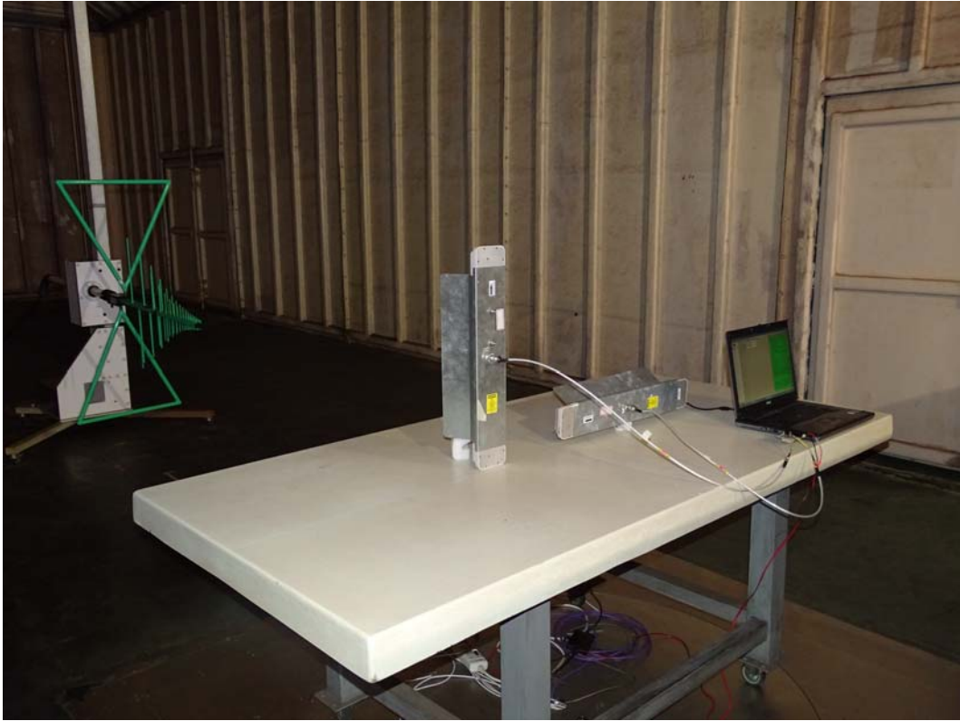
Front View of Radiated Test (Sector Antenna)
