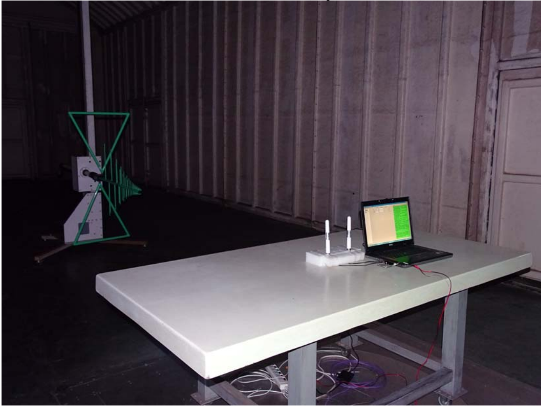
Front View of Radiated Test (Dipole Antenna)
