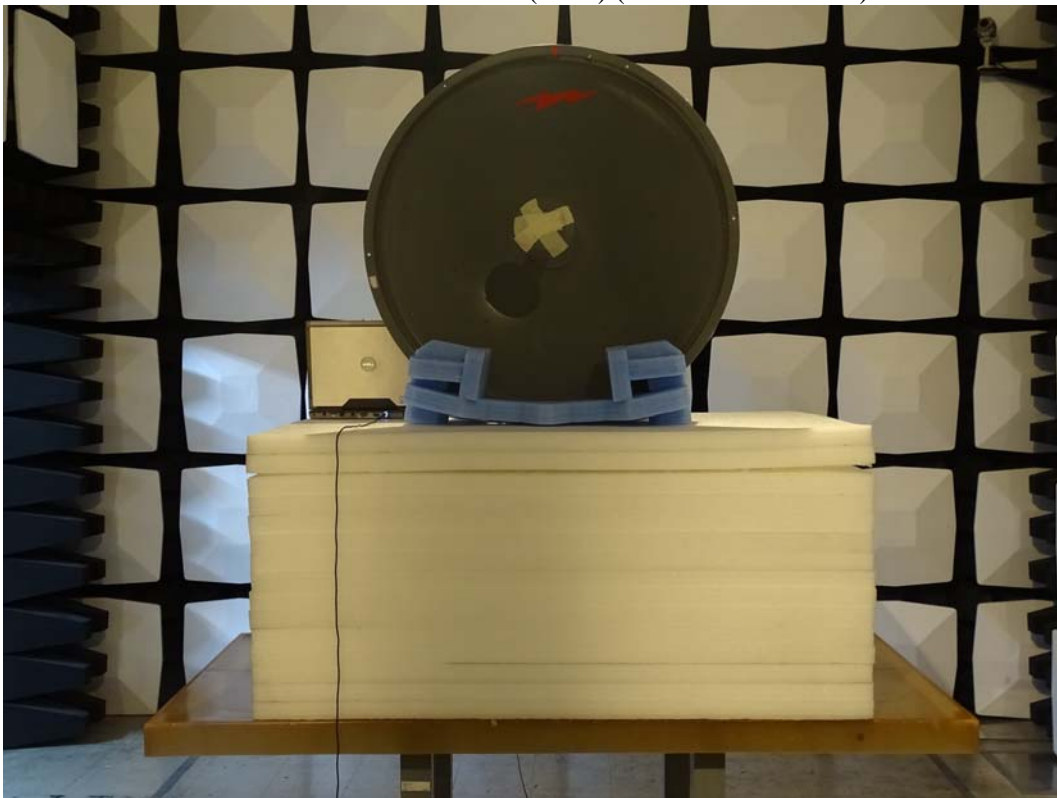
Back View of Radiated Test (Horn) (Grid DISH Antenna)
