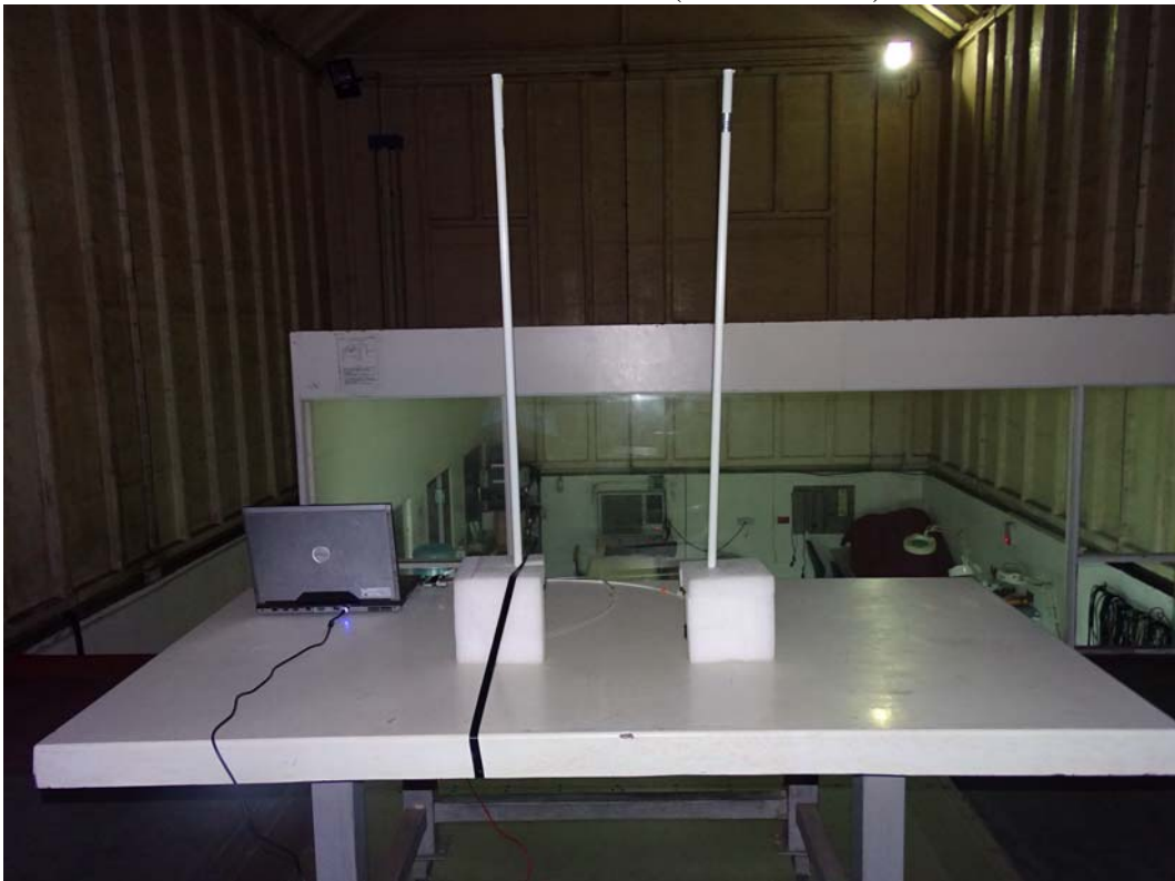
Back View of Radiated Test (Omni Antenna)
