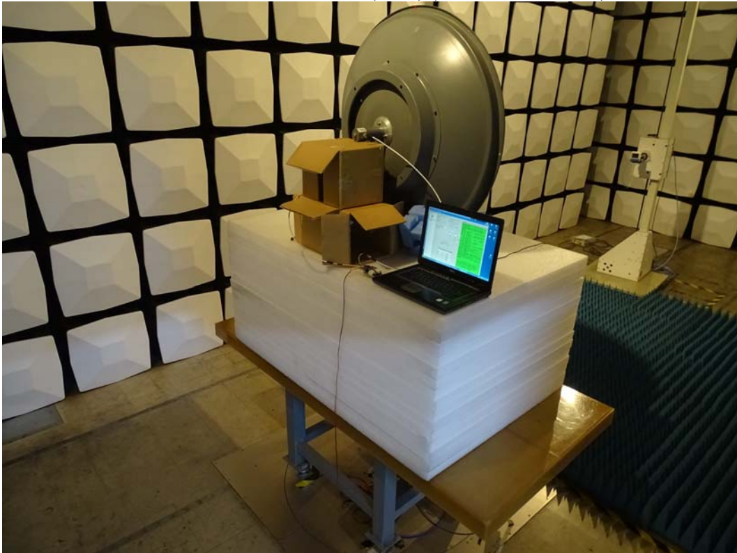
Front View of Radiated Test (Horn) (Grid DISH Antenna)
