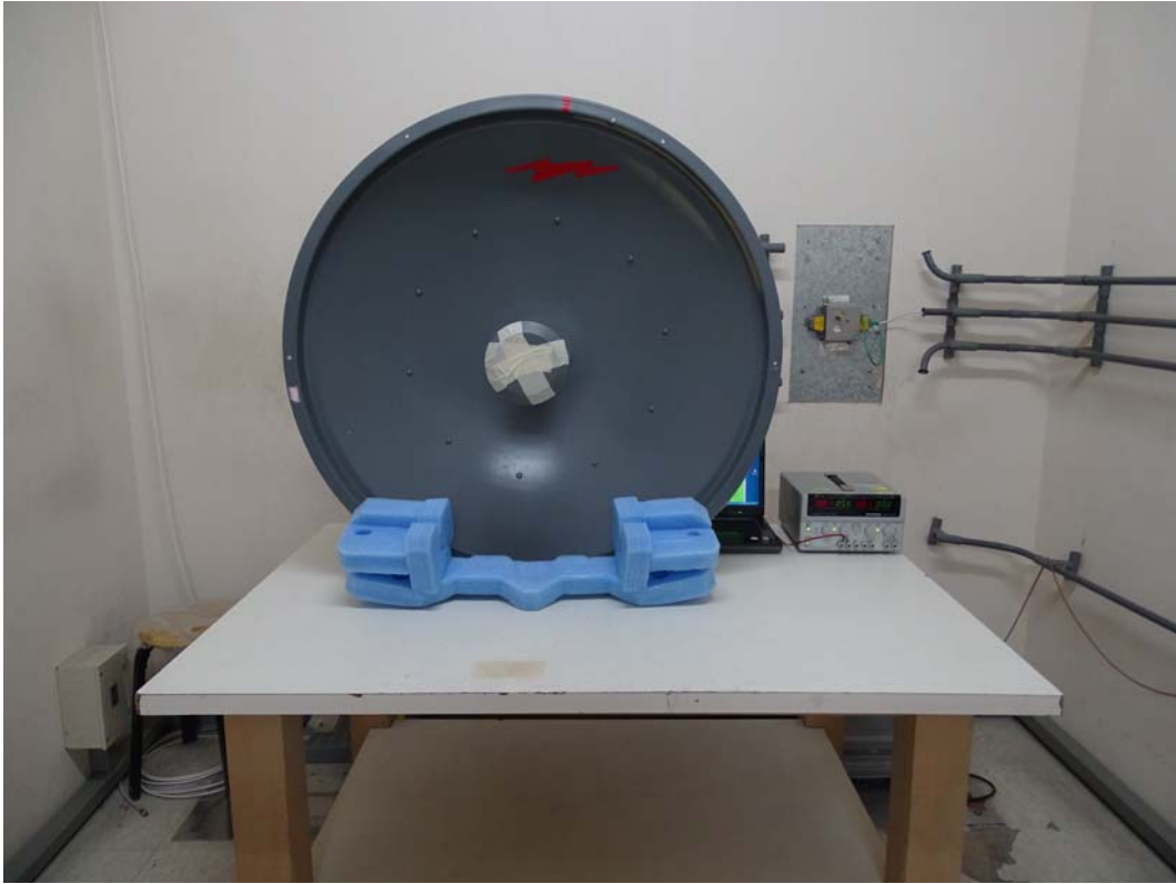
Front View of Conducted Test (Grid DISH Antenna)
