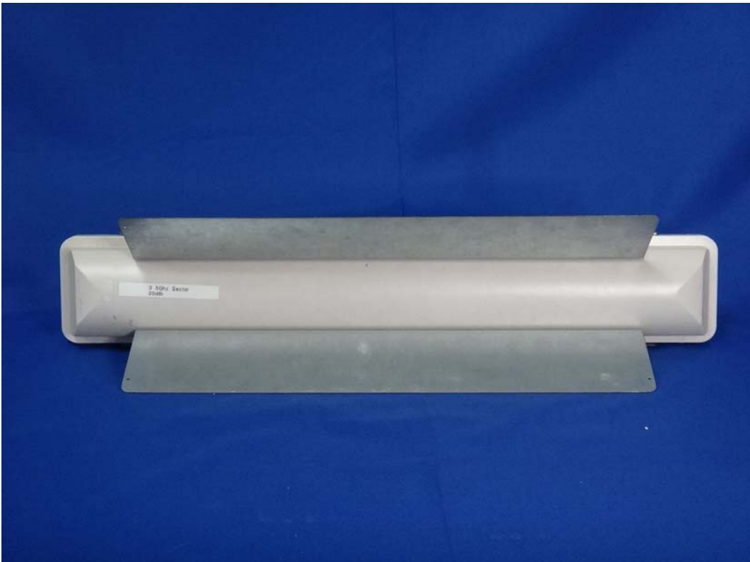
(12) EUT Photo (Sector Antenna)
