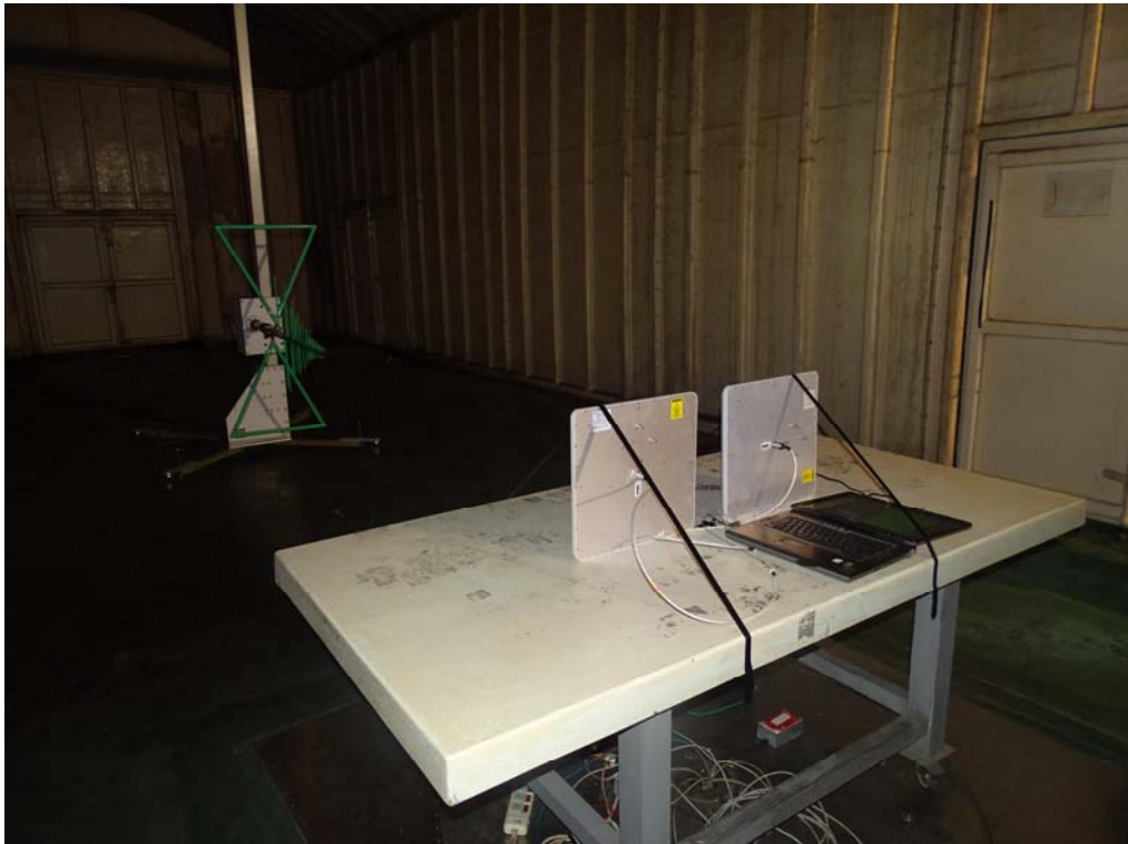
Front View of Radiated Test-Panel
