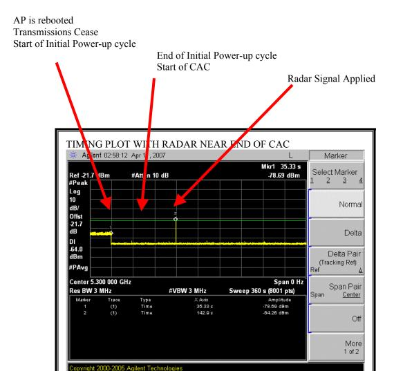
The radar signal is applied (142.9 - 35.33) = 107.54 seconds after reboot, which is (107.54 - 48.08) = 59.46 seconds after the start of the CAC period.
