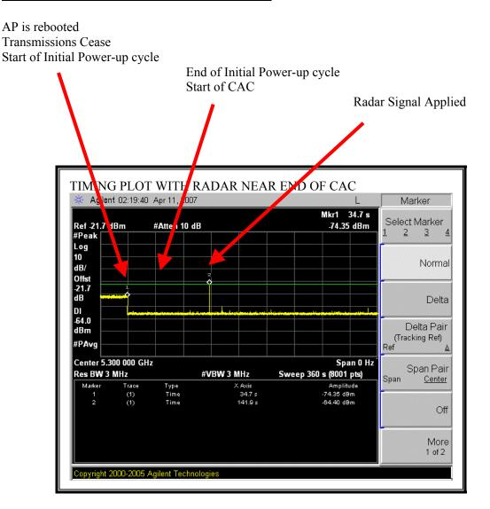
The radar signal is applied (141.9 - 34.7) = 107.2 seconds after reboot, which is (107.2 - 49.09) = 58.11seconds after the start of the CAC period.
