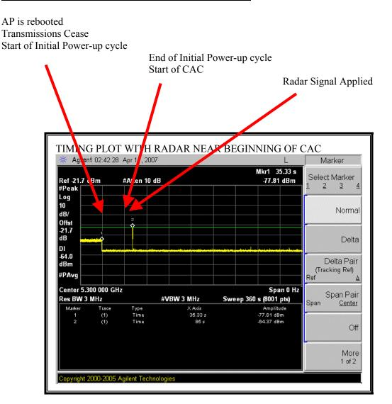
The radar signal is applied (85 - 35.33) = 49.67 seconds after reboot, which is (49.67 - 48.08) = 1.59 seconds after the start of the CAC period.
