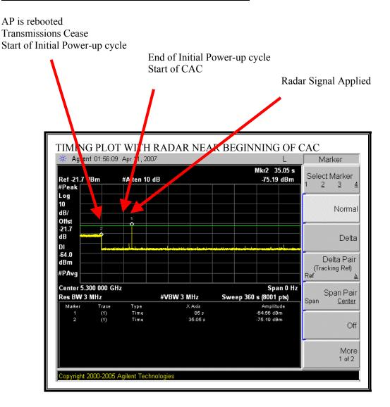
The radar signal is applied (85 - 35.05) = 49.95 seconds after reboot, which is (49.95 - 49.09) = 0.9seconds after the start of the CAC period.
