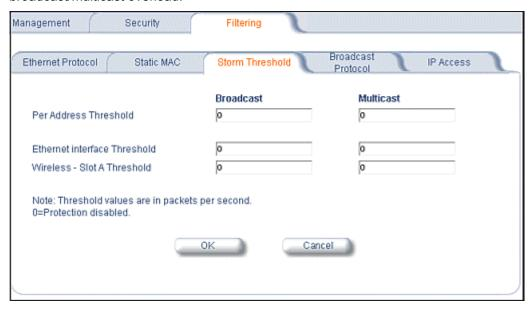
Storm Threshold is an advanced **Bridge** setup option that you can use to protect the network against data overload by specifying:
