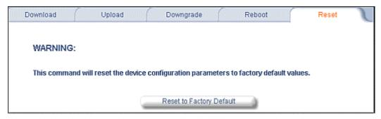
You can also reset the MP.11/a from the RESET button located on the side of the unit. Because this resets the MP.11/a's current IP address, a new IP address must be assigned.
