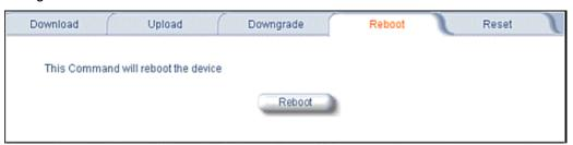
CAUTION: Rebooting the unit causes all users currently connected to lose their connection to the network until the MP.11/a has completed the restart process and resumed operation.
