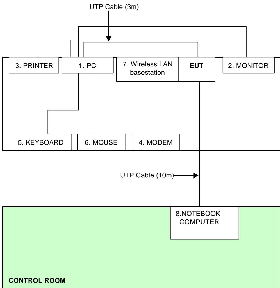
**NOTE:** 1. Support unit 8 was kept in the control room during the test.
