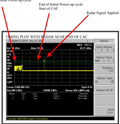
The radar signal is applied (135.7 - 35.23) = 100.47 seconds after reboot, which is (100.47 - 43.21) = 57.26 seconds after the start of the CAC period.
