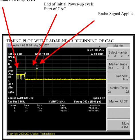
The radar signal is applied (82.25 - 34.74) = 47.51 seconds after reboot, which is (47.51 - 43.21) = 4.3 seconds after the start of the CAC period.
