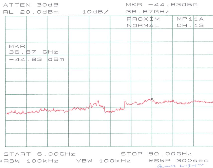
*Plots of Spurious Emission for 5250-5350MHz Band (15.407)*
