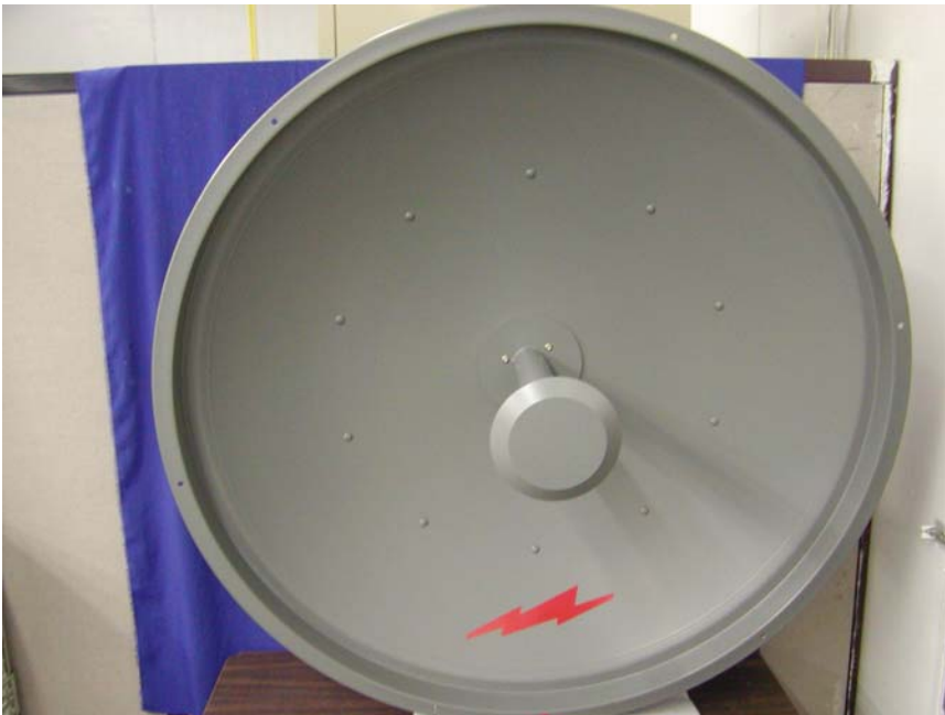
P3F-52-N7A Dish Antenna – Front View
