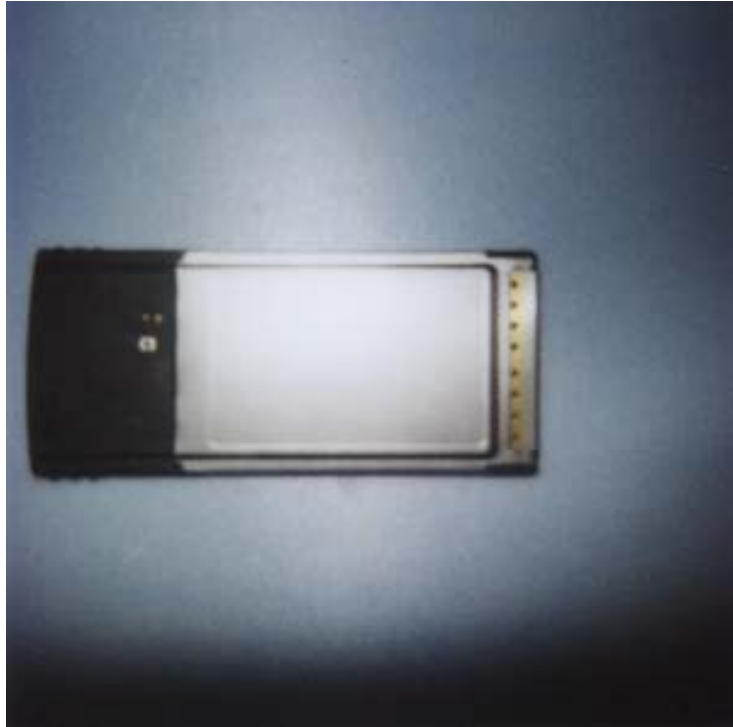
Fig. 11. Photograph of the Proxim Europe B.V. Model 8460-05 Cardbus Card with coaxial output for conducted power measurements.
