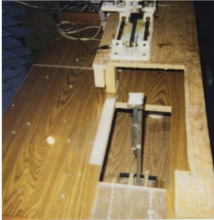
Fig. 4. The plastic holder used to support the portable computer with the Proxim Europe B.V. Model 8460-05 Cardbus Card (shown in Fig. 1).
