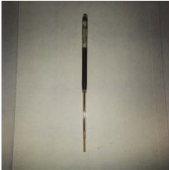
Fig. 7. Photograph of the Narda Model 8021 Broadband Electric Field Probe used for SAR measurements.
