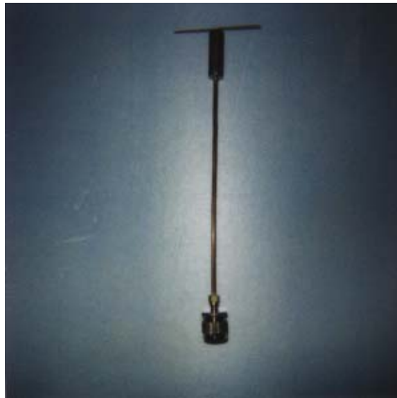
Fig. 8. Photograph of the half-wave dipole at 1900 MHz used for system verification.
