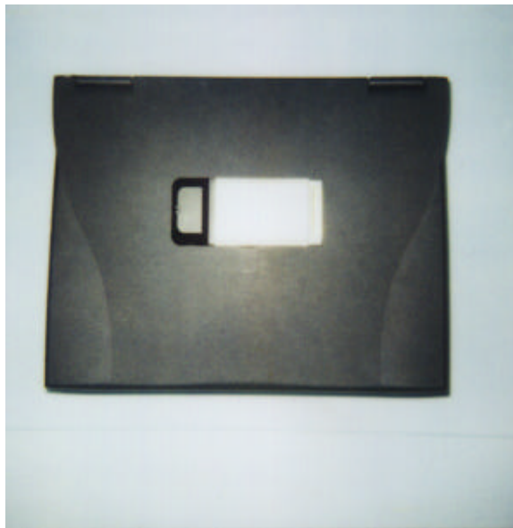
Fig. 2. A picture of the Proxim Model 8460 CardBus Card placed on the laptop computer.
