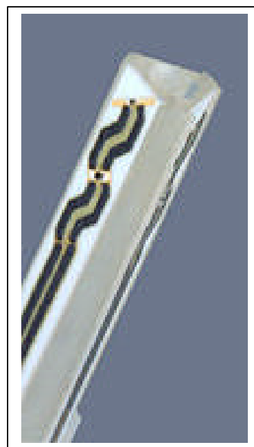
Inside view of ET3DV6 E-field Probe
