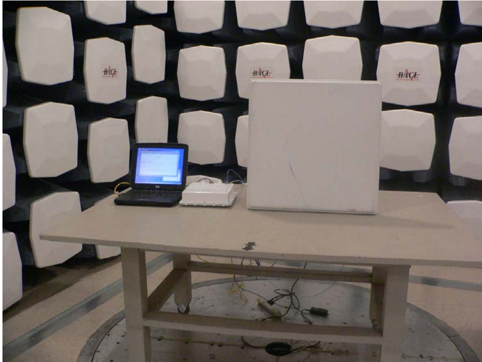
Radiated Emission – Front View (Panel Antenna 28.5 dBi )
