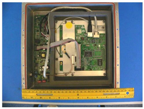
EUT Cover Off With the Filter Board
