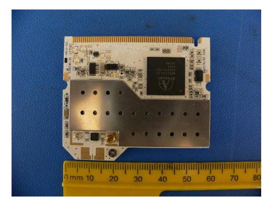
**RF Board with Shield Off – Front**
