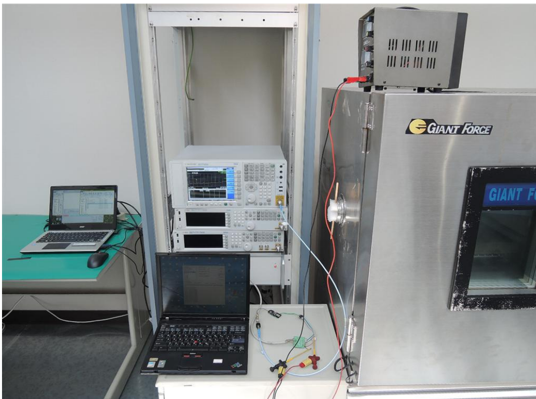
Photograph 4: Set-up for Conducted testing
