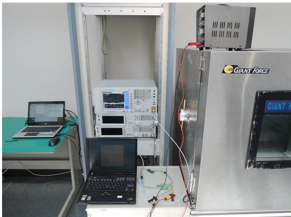
Photograph 4: Set-up for Conducted testing
