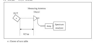
Distance Factor: 20 x log  $(0.5 \text{ m}^* / 3.0 \text{ m}) = -15.6 \text{ dB}$ \*Test Distance: 0.5 m
