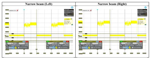
The declared duty factor and measured one were compared. The maximum duty factor of these results was applied to the average field strength measurement. (Worst case)
