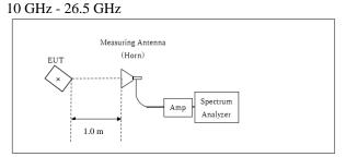
Distance Factor: 20 x log  $(3.75 \text{ m}^*/3.0 \text{ m}) = 1.94 \text{ dB}$ \* Test Distance: (3 + SVSWR Volume /2) - r = 3.75 m
