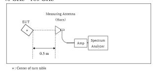
Distance Factor: 20 x log (0.5 m\* / 3.0 m) = -15.6 dB \*Test Distance: 0.5 m
