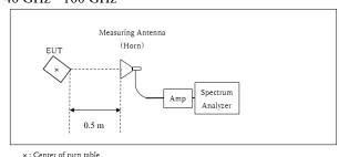
Distance Factor:  $20 \times \log (0.5 \text{ m}^* / 3.0 \text{ m}) = -15.6 \text{ dB}$  \*Test Distance: 0.5 m
