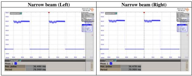
The declared duty factor and measured one were compared. The maximum duty factor of these results was applied to the average field strength measurement. (Worst case)
