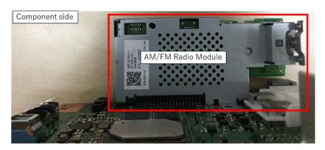
The AM/FM connector is shown in the red frame in the figure.
