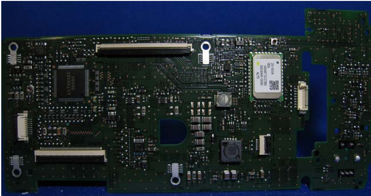
PCB including Bluetooth IC (Component Side)
