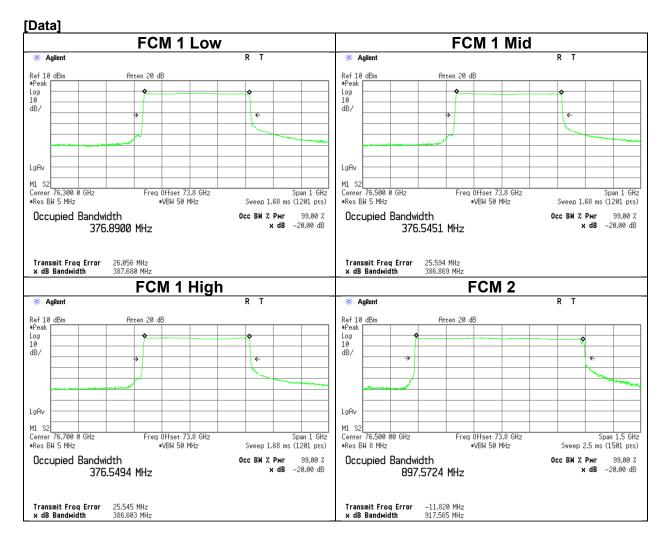
The measurement was performed with Peak detector and Max Hold since the duty cycle was not 100 %.
