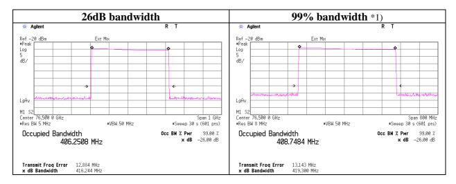
\*1) The measurement was performed with Peak detector, Max Hold since the duty cycle was not 100%.
