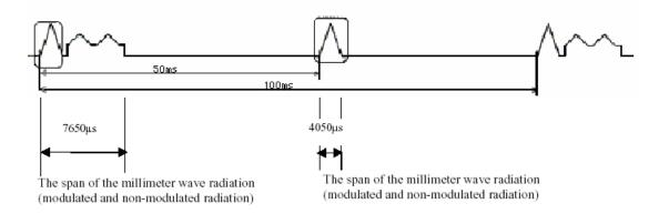
The total ON time is 11.7 msec within a 100 msec period. This yields a duty cycle of 11.7% and a correction factor of -9.32 dB.
