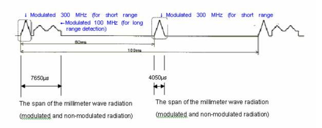
The correction factor is calculated with  $10 \log (TX \text{ on} / 100 \text{ ms})$  here -9.3 dB
