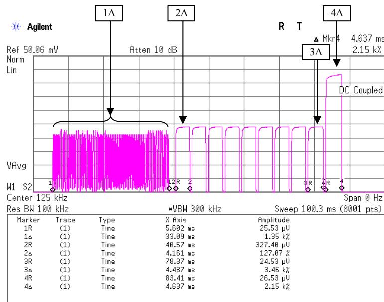
Only 4Δ is simultaneous transmission from two antennas.
