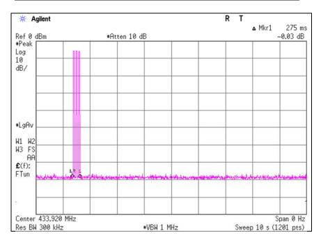
\* The EUT transmits UHF when LF signal is received from a car or a button on the EUT is pressed. In both cases, the UHF transmission is stopped within 5 seconds. So the test was performed by a button-pressed operation as the worst case. Please refer to the "Theory of Operation" for details.
