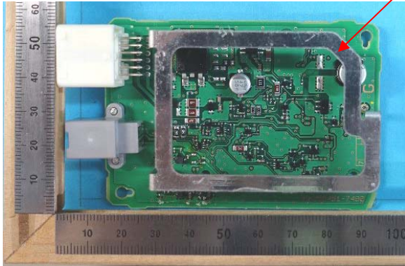
Component side with antenna
