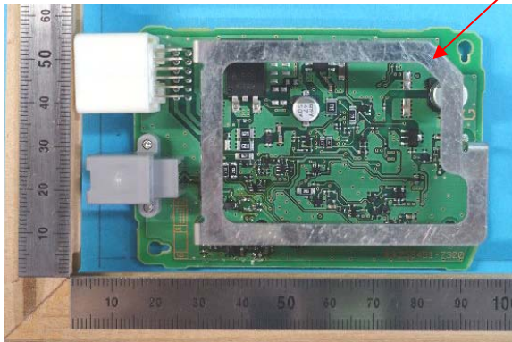
Component side with antenna
