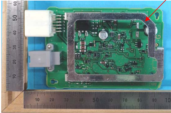
Component side with antenna
