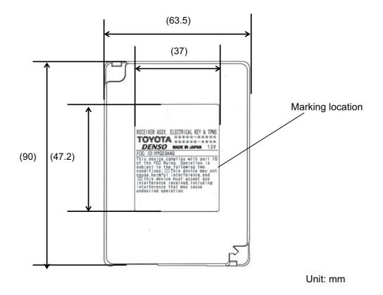
Fig. Marking location and Appearance of Receiver
