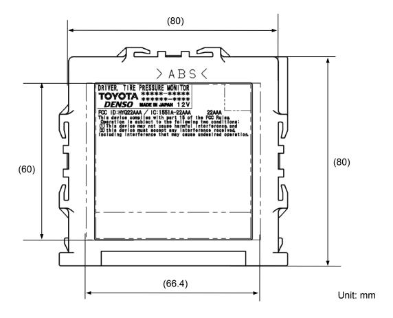
Fig. Marking location and layout of Driver
