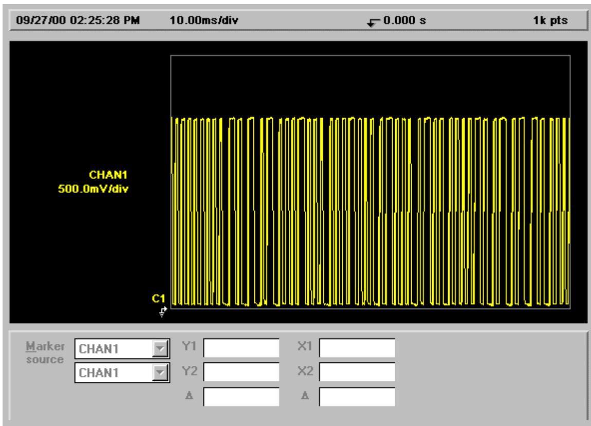
11 wide pulses and 41 narrow pulses,  $11(1.625 \text{ msec}) + 41(.8 \text{ msec}) = 49.875 \text{ msec}$
