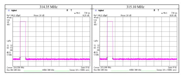
\* The EUT transmits UHF when LF signal is received from a car or a button on the EUT is pressed. In both cases, the UHF transmission is stopped within 5 seconds. So the test was performed by a button-pressed operation as the worst case.
