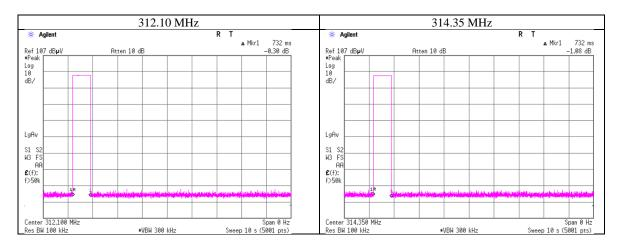
\* The EUT transmits UHF when LF signal is received from a car or a button on the EUT is pressed. In both cases, the UHF transmission is stopped within 5 seconds. So the test was performed by a button-pressed operation as the worst case. Please refer to the "Theory of Operation" for details.
