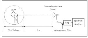
Distance Factor:  $20 \times \log (4.0 \text{ m} / 3.0 \text{ m}) = 2.50 \text{ dB}$ \* Test Distance: (3 + SVSWR Volume /2) - r = 4.0 m
