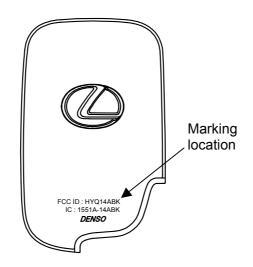
Fig. Marking location and layout of Transmitter
