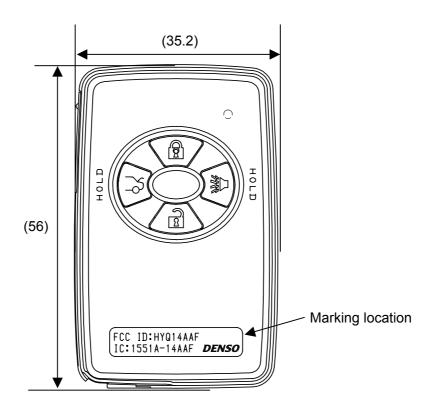
Fig. Marking location and layout of Transmitter
