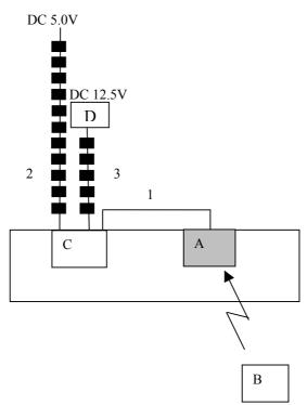
: Standard Ferrite Core (EUT noise were not influenced by these ferrite cores)
