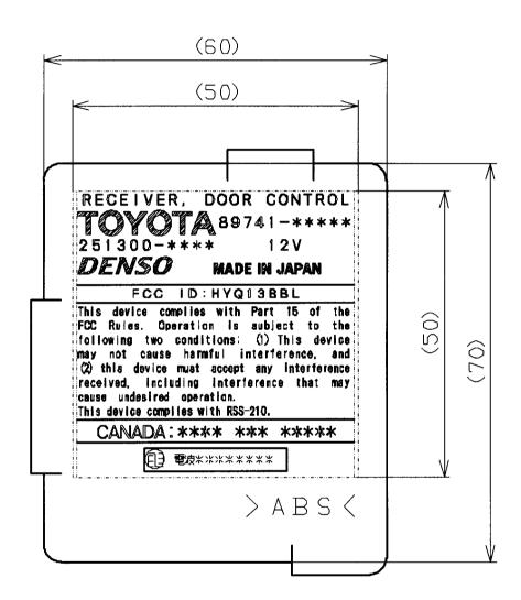
Fig. Marking location and layout of receiver
